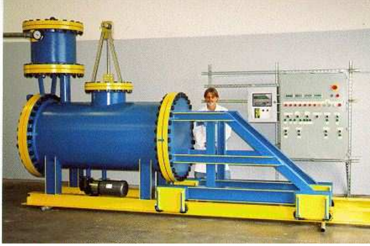
Figure 14. Picture of a 250 Kw Santilli's Hadronic Reactor (also called PlasmaArcFlow Reactor) with the panels of its completely automatic and remote controls, to recycle liquid waste into magnegas usable for any fuel application, a large amount of heat and carbonaceous precipitates used to produce the electrodes. This Reactor can produce up to 5000,000 scf (140 millions liters) of magnegas per week of 24 hours work per day corresponding to 3,000 gasoline gallon equivalent (11,000 gasoline liter equivalent) of magnegas per week computed on the basis that: 1) Gasoline contains about 110,000 BTU/g (about 29,000 BTU/liter); 2) Magnegas has the low energy content of 750 BTU/scf (26 BTU/liter); and 3) the "gasoline gallon equivalent" is given by about 150 scf of magnegas ("gasoline liter equivalent" is given by about 29 liters of magnegas). PlasmaArcFlow reactors are completely self-contained. Consequently, they release no solid, liquid or gas to the environment and cause no noise or odor pollution (see website [5b] for details).
