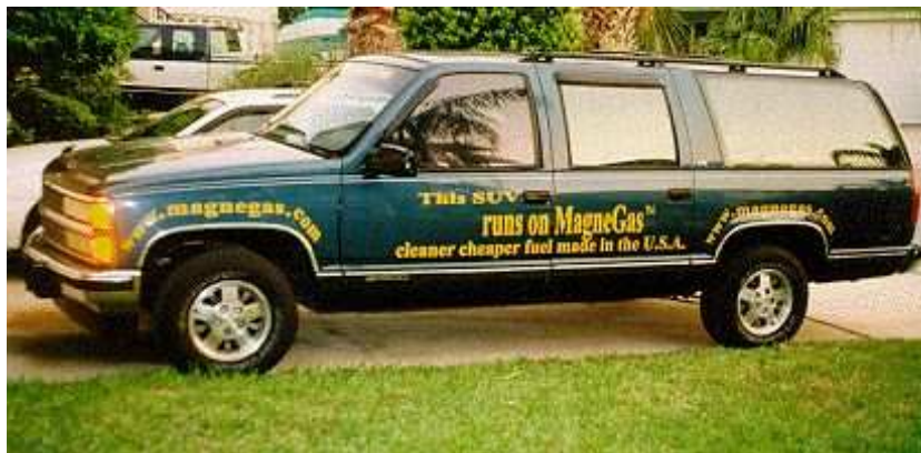
Figure 17. A picture of a Chevrolet Suburban SUV 1992 converted by the author to operate as a bifuel gasoline/magnegas with a switch on the dashboard permitting to pass from one fuel to the other while driving. Bifuel cars are produced by numerous carmakers to operate on gasoline and natural gas. The same cars can operate on magnegas (in place of natural gas) with the sole adjustment of the pressure regulator to optimize the stoichiometric ratio air/fuel, since the latter for magnegas is much smaller than that for natural gas because magnegas is very rich internally in oxygen, thus requiring a fraction of the air needed by natural gas to operate. These bifuel cars are ideally suited for the magnegas technology because, when magnegas runs out, one can still reach the magnegas refilling station on gasoline (see website [5b] for details).
