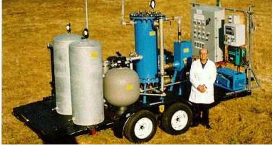
Figure 15. Picture of a 50 Kw Santilli's Hadronic Reactor (PlasmaArcFlow Recycler) mounted on a trailer for mobility to conduct test recycling where liquid wastes are located. This recycler can produce up to 84,000 scf (up to 2.4M liters) of magnegas per week corresponding to about 560 gasoline gallon equivalent (2,100 gasoline liter equivalent) of magnegas per week (see website [5b] for details).
