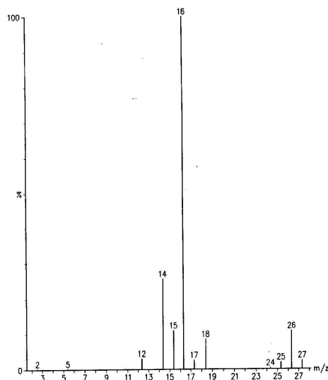
Figure 52. The scan conducted by SunLabs on the HHO gas detecting a peak at 16 amu that confirms the presence of atomic oxygen in the HHO gas of Fig. 51, plus a peak at 17 amu indicating the presence of traces of the radical O-H , a peak at 18 amu indicating the presence of water vapor all three species also detected in the scan of Fig. 51, as well as additional anomalous peaks at 12, 14, 25, 26, 27 amu that, for the case of the HHO gas produced from distilled water cannot admit a molecular interpretation.
