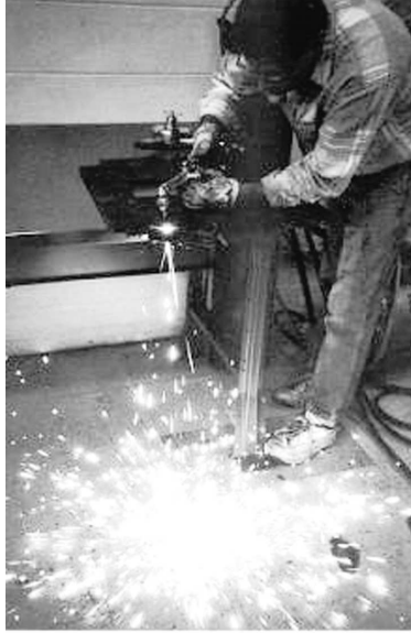
Figure 34. A view of metal cutting via magnegas. Independent certifications by various users have established that: 1) magnegas has a pre-heat time at least half that by acetylene (which is currently used for metal cutting and has an energy content of 2,300 BTU/cf); 2) magnegas cuts metal at least 50% faster than acetylene; 3) the cut produced by magnegas is much smoother without edges as compared to that by acetylene; 4) magnegas exhaust does not contain carcinogenic or other toxic substances, while that of acetylene is perhaps the most carcinogenic and toxic of all fuels; 5) magnegas cutting does not produce the “flash-back” (local explosion of paint over metal) typical of acetylene; 6) magnegas is dramatically safer than acetylene, which is unstable and one of the most dangerous fuels currently used; and 7) magnegas cost about 1/2 that of acetylene.
