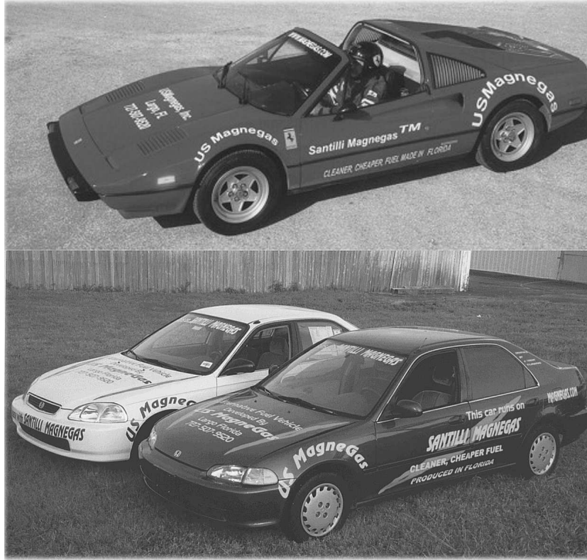
Figure 16. A picture of a Ferrari 308 GTSi 1980 and two Honda Civic cars converted by the author to operate with the new clean burning magnegas without catalytic converter, yet surpassing all EPA exhaust requirements, having no carcinogenic or other toxic substance in the exhaust, reducing of about 50% the \text{CO}_2 emission due to gasoline combustion, reducing the operating temperature of about 25%, and emitting in the exhaust 10% to 14% breathable oxygen (see website [5b] for details).
