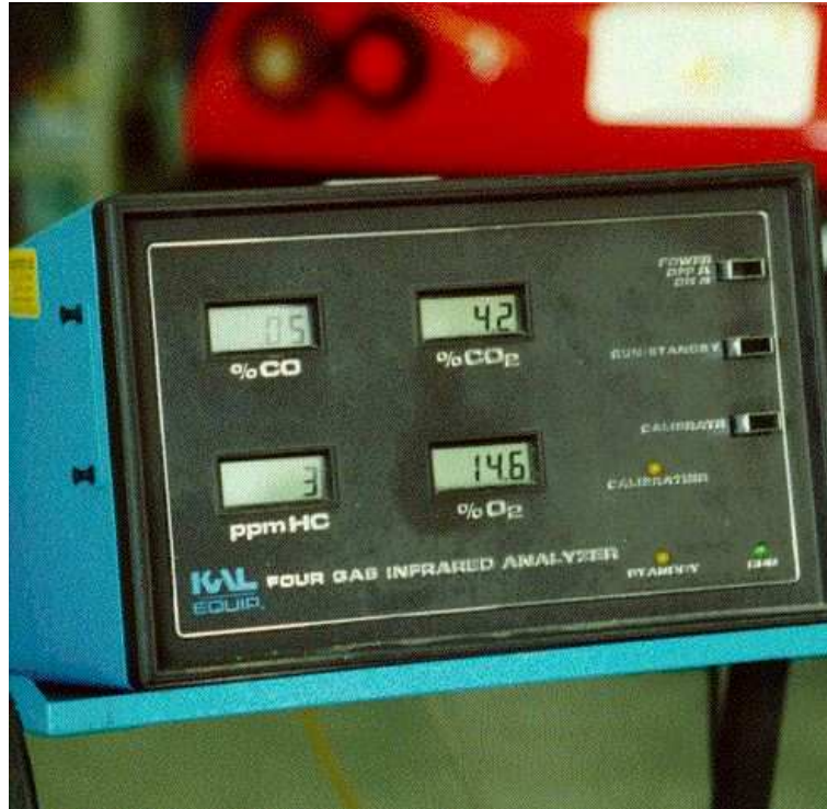
Figure 19. A picture of the readings of a 4-ways exhaust analyzer testing the exhaust of the Ferrari 308 GTSi of a preceding picture operating on magnegas “without” catalytic converter. Note: the presence of 14% breathable oxygen in the exhaust; about half the \text{CO}_2 produced by the same car when running on gasoline; the very few detected hydrocarbons originate from engine oil seeping through the piston rings because magnegas “cannot” contain hydrocarbons since it is synthesized at the 5,000^\circ\text{C} of the arc at which temperature no hydrocarbon can survive; the very small content of CO in the exhaust is due to poor combustion because CO is fuel for magnegas, while it is a byproduct of the combustion for fossil fuels, as a result of which detecting CO in the exhaust of a car running on magnegas is the same as detecting gasoline in the exhaust of a car running on gasoline (see website [5b] for details).
