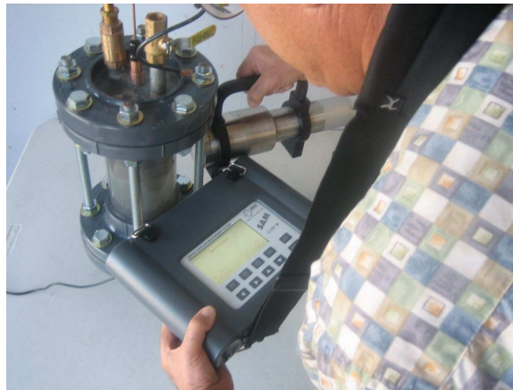
Figure 1: A picture of Klystron I and of detector SAM 935. Note the similarity with the klystron used in tests [3], but also the primary differences being given by the use of metal walls for Don Borghi's tests, and transparent polycarbonate walls for Santilli's tests. The latter were selected so as to permit the visual identification of the creation of an interior electric arc with a gap between the electrodes, the latter being necessary to assure the creation of a discharge through the hydrogen gas in which absence all tests are invalid.
